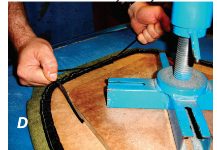
Compress Foam and pull cord
