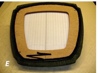
Staple excess cord to Seat board
