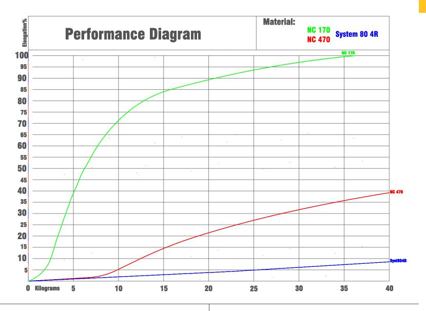
The graph shows the tensile/elongation curve for typical Matrex webbings. In this instance, it shows the application tension for NC 1 50 elongation 100%, NC 470 elongation 40%, and Systems 80 elongation 6%. As a load is applied, the webbing stretches to its optimum elongation and maintains an elastic range that provides resiliency. Our construction prevents further sagging or bottoming out.
